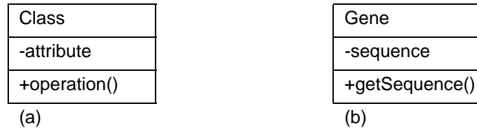
Figure A.2 (a) Schematic for a UML class (b) Simple Gene class
